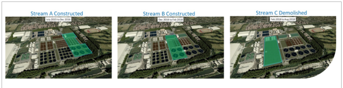
Figure 15 - Illustration of the progressive upgrade on site during full operation
